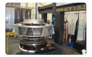
Cruiser series CMM offers maximum measurement volume for large work-pieces. Advanced means and methods which are designed by professional software, analyzed by finite element and dynamic property etc ensure measuring high stability and accuracy.
